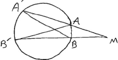
$\begin{cases} \widehat{A}' = \frac{1}{2}AB \\ \widehat{B}' = \frac{1}{2}AB \end{cases} \rightarrow \widehat{A}' = \widehat{B}'$ $(\widehat{A}' = \widehat{B}'), (M = M) \rightarrow \Delta MA'B \sim \Delta MB'A \rightarrow \frac{MA}{MB} = \frac{MB'}{MA'} \rightarrow MA \cdot MA' = MB \cdot MB'$ |
