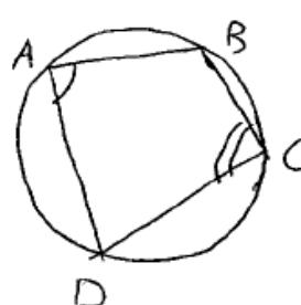
$\begin{aligned} \widehat{A} + \widehat{C} &= \frac{1}{2} BCD + \frac{1}{2} BAD \\ &= \frac{1}{2} (BCD + BAD) = \frac{1}{2} (360^\circ) = 180^\circ \end{aligned}$                                                                                                                                   |
